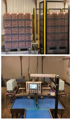
A ROBOT PICKS UP FOUR STACKS AT A TIME, INSERTS A DIVIDE BETWEEN EACH LAYER, AND EVENTUALLY FILLS THE WHOLE PALLET
